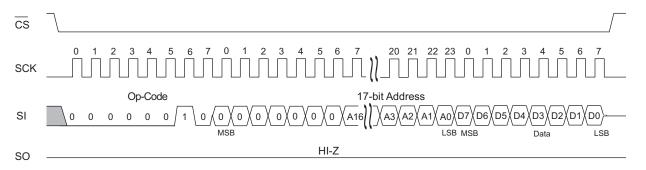
Figure 13. Burst Mode Write Instruction Timing
